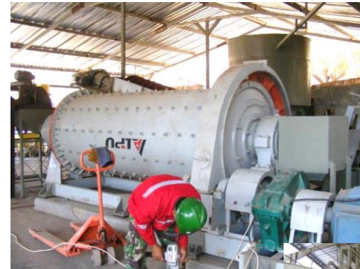
Ball mill – 3.0m x 1.2m 200 mesh (75 micron) output
